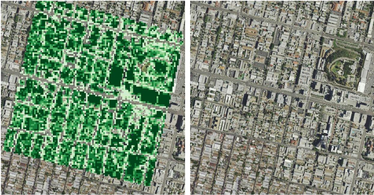
Figure 2.—Example of the LiDAR dataset (left) metric for 1<sup>st</sup> returns above 2m in height (Pct1stRtns) identifying structures on the landscape. The image on the right is NAIP 2011 imagery.
